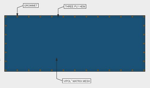
weld and one row of black UV treated thread at the center of the screen. They include grommets every 12".
